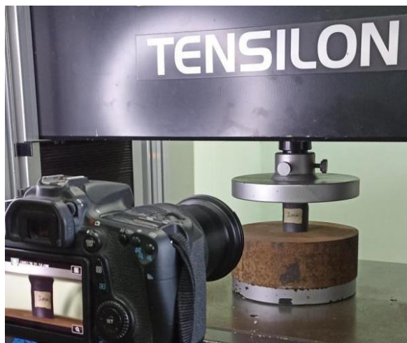
Figure 2. The experimental setup for quasi-static compression testing
