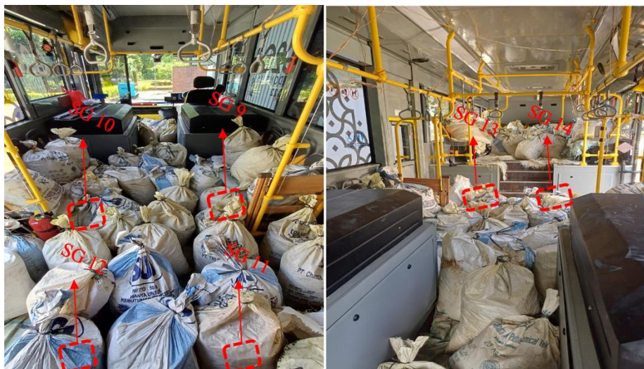
Figure 16. Strain gauge at central deck
