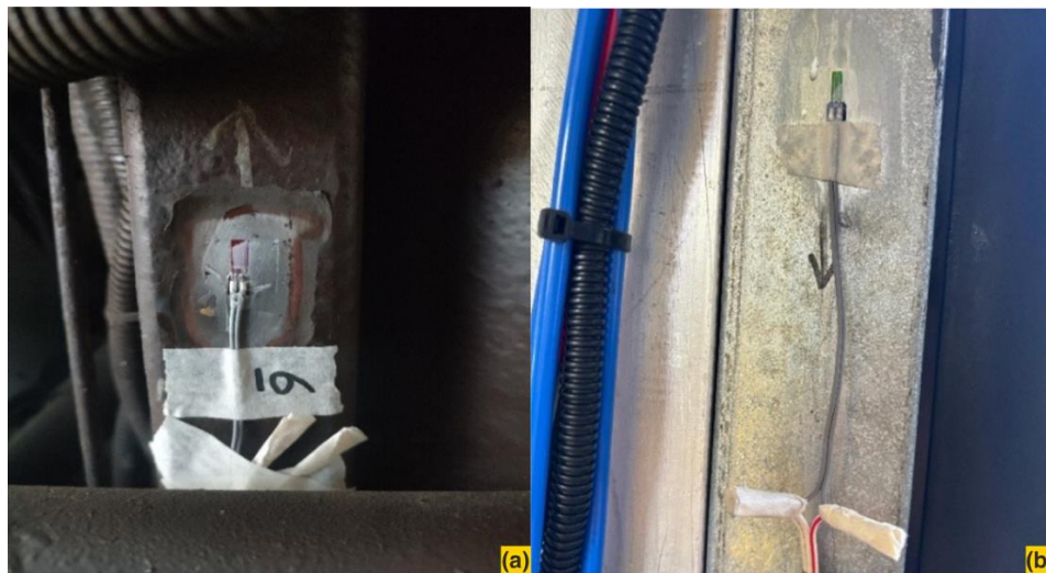
Figure 6. (a) Strain gauge on lower frame; (b) Strain gauge on upper frame
