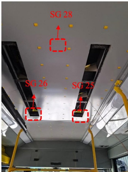
Figure 17. Strain gauge at air conditioning system
