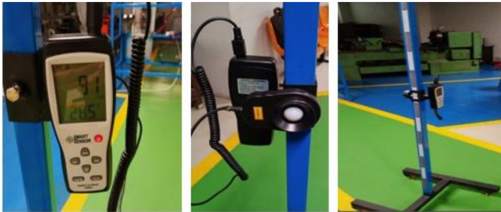
Figure 14. Light intensity in lux is measured with a lux meter
