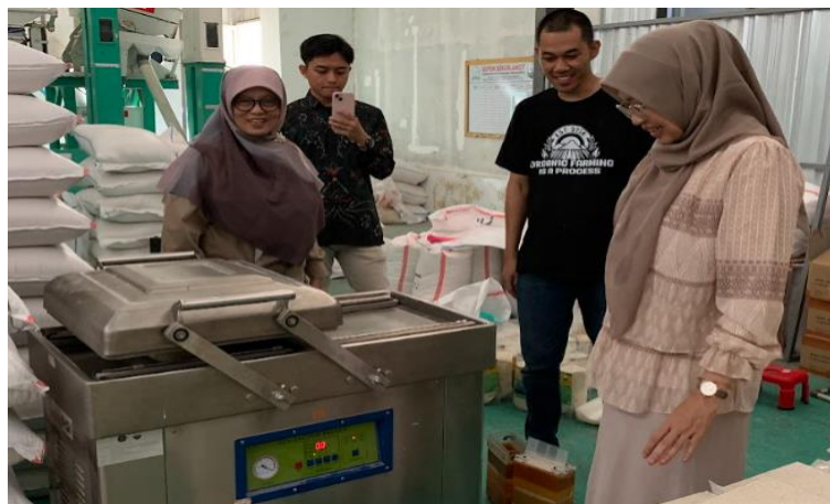
Gambar 3. Praktik penerapan mesin vaccum double chamber
